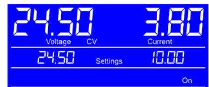
The manual adjustment of the set values can only be done while the device is not in a different mode, like adjustment mode for OVP/OCP values. See figure to the right. In normal operation mode, the middle row shows the set values.
